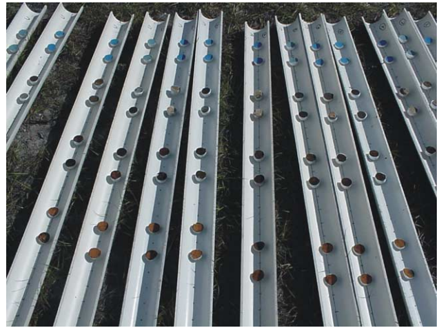
Photograph 1. Sliding coupon holder with biofilm coupons
